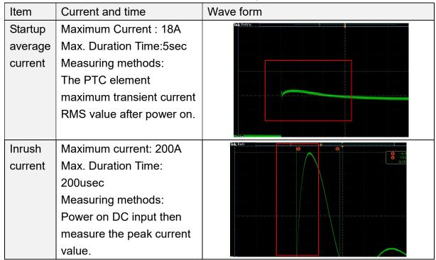
Table 2-1. Tested waveform to startup average current and inrush current.
