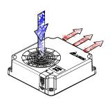
\*Note A. Mimum gap for air inlet and exit is required to avoid the damage caused from blocked air passage
