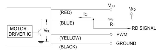
CAUTION: THE RD SIGNAL LEAD WIRE MUST BE KEPT AWAY FROM"+" LEAD WIRE & "-" LEAD WIRE.
