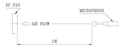
NOISE IS MEASURED AT RATED VOLTAGE IN FREE AIR IN SEMI-ANECHOIC CHAMBER WITH MICROPHONE AT A DISTANCE OF ONE METER FROM THE FAN INTAKE.
