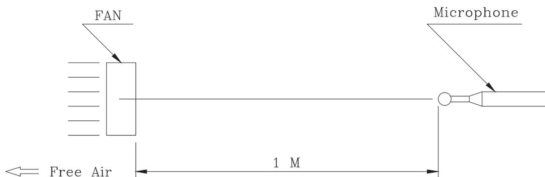
NOISE IS MEASURED AT RATED VOLTAGE IN FREE AIR IN ACOUSTICAL CHAMBER WITH B & K SOUND LEVEL METER.
