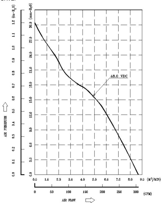
\*TEST CONDITION: INPUT VOLTAGE-----OPERATION VOLTAGE
