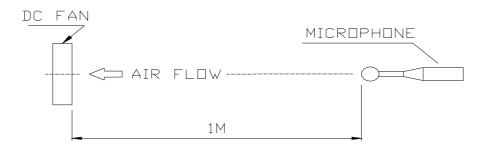
DOISE IS MEASURED AT RATED VOLTAGE IN FREE AIR IN ANECHOIC CHAMBER WITH B & K SOUND LEVEL METER WITH MICROPHONE AT A DISTANCE OF ONE METER FROM THE FAN INTAKE.
