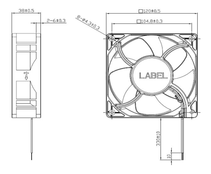
LEAD WIRE: UL 3266 AWG #24 125°C/ 300V
