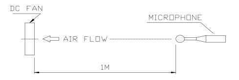
NOISE IS MEASURED AT RATED VOLTAGE IN FREE AIR IN SEMI-ANECHOIC CHAMBER WITH B & K SOUND LEVEL METER WITH MICROPHONE AT A DISTANCE OF 1M FROM THE FAN INTAKE.
