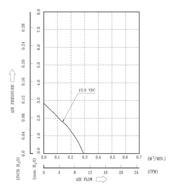
\*TEST CONDITION: INPUT VOLTAGE-----OPERATION VOLTAGE
