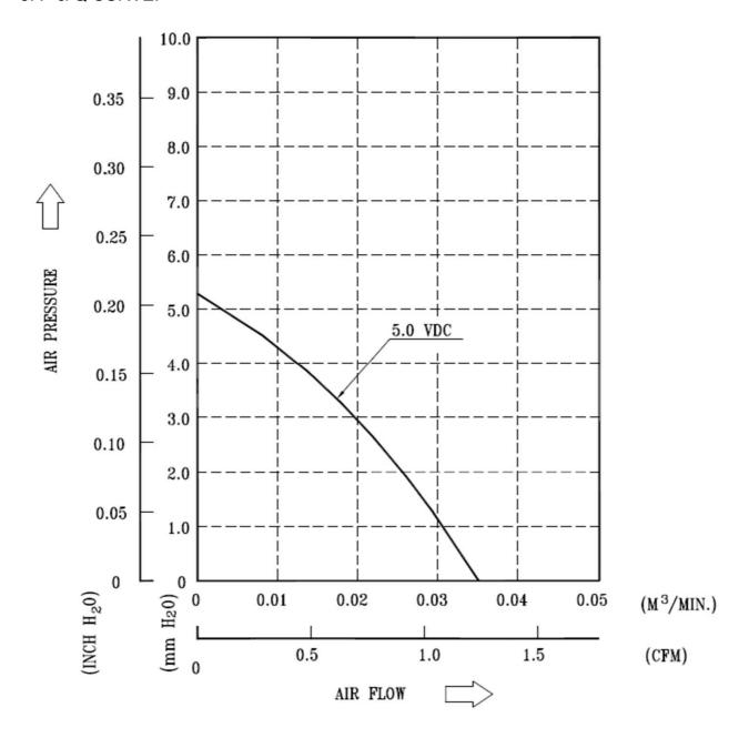
\*TEST CONDITION: INPUT VOLTAGE-----OPERATION VOLTAGE
