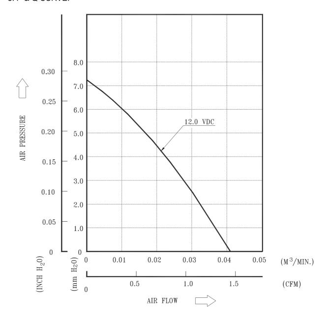
\*TEST CONDITION: INPUT VOLTAGE-----OPERATION VOLTAGE
