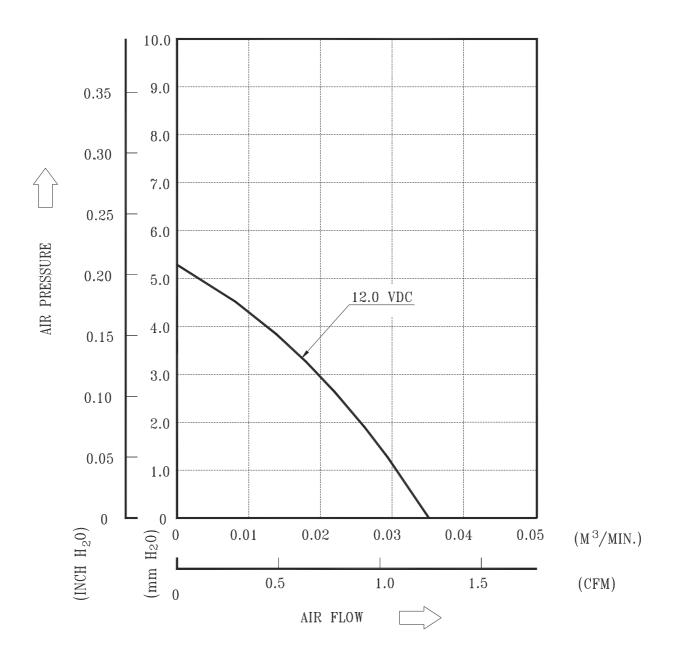
\*TEST CONDITION: INPUT VOLTAGE-----OPERATION VOLTAGE
