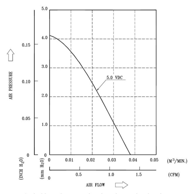
\*TEST CONDITION: INPUT VOLTAGE-----OPERATION VOLTAGE
