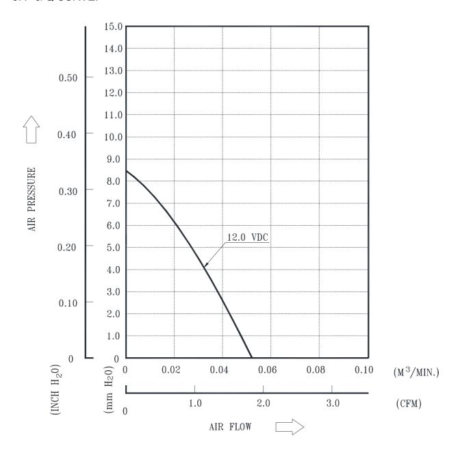
\*TEST CONDITION: INPUT VOLTAGE-----OPERATION VOLTAGE
