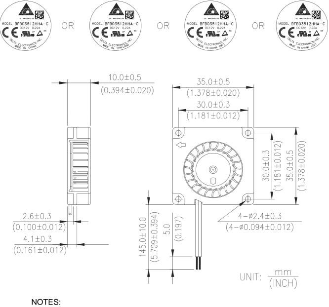
1. LEAD WIRE: UL 1571 AWG #30 RED WIRE-----(+) BLACK WIRE-----(-)
