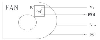
SIGNAL VOLTAGE RANGE:  $0 \sim (V_+ - 0.5)$  VDC
