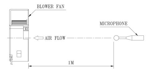
NOISE IS MEASURED AT RATED VOLTAGE IN FREE AIR IN SEMI-ANECHOIC CHAMBER WITH MICROPHONE AT A DISTANCE OF ONE METER FROM THE FAN INTAKE.
