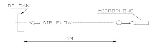
NOISE IS MEASURED AT RATED VOLTAGE IN FREE AIR IN ANECHOIC CHAMBER WITH B & K SOUND LEVEL METER WITH MICROPHONE AT A DISTANCE OF ONE METER FROM THE FAN INTAKE.
