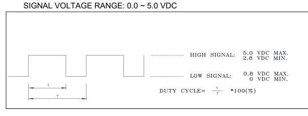
\*THE PREFERRED OPERATING POINT FOR THE FAN IS 25KHz. \*AT 100% DUTY CYCLE, THE ROTOR WILL SPIN AT MAXIMUM SPEED. \*AT 0% DUTY CYCLE, THE ROTOR WILL WILL SPIN AT MINIMUM SPEED \*WITH CONTROL SIGNAL LEAD DISCONNECTED, THE FAN WILL SPIN AT MAXIMUM SPEED.
