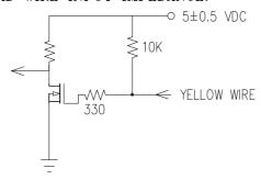
13-1. THE FAN SPEED WILL DEFAULT TO MAXIMUM WHEN THE SPEED CONTROL INPUT IS LEFT UNCONNECTED.
