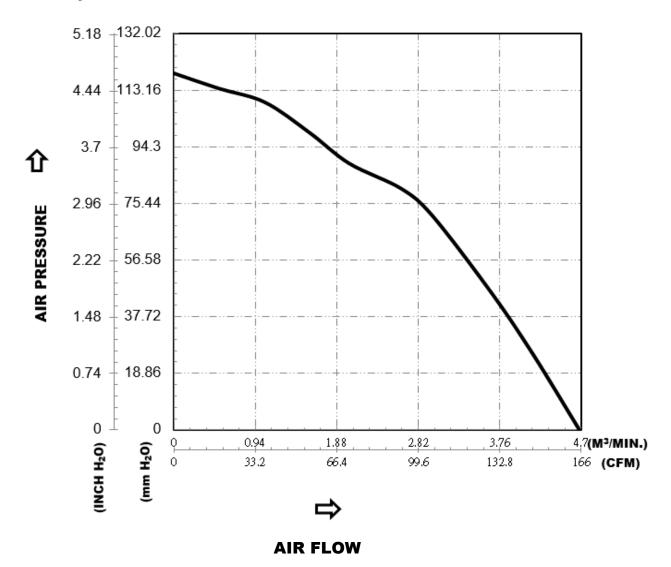
\*TEST CONDITION: INPUT VOLTAGE-----OPERATION VOLTAGE
