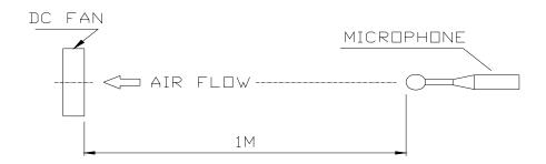
NOISE IS MEASURED AT RATED VOLTAGE IN FREE AIR IN SEMI-ANECHOIC CHAMBER WITH MICROPHONE AT A DISTANCE OF ONE METER FROM THE FAN INTAKE.
