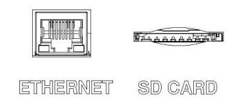
The controller used communication technology to remotely control, monitor, SD card 8 GB for logging data and alarm the cooling function of the ACU. This can be done using a RJ45 or RS485 connected to an industrial network or a personal computer (PC) connected to an Internal local area network.
