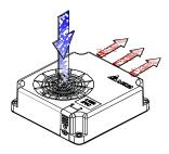
\*Note A.Mimum gap on both cool air inlet and warm air outlet to avoid warm have standstill to affect mechanical thermostat and cutoff thermo fuse judgement and cause higher temperature to damage the heater.
