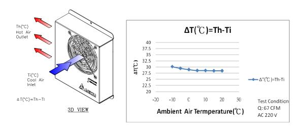
\*Note A. Minimumgapisrequiredoninletandexitpassagetoavoidtriggertheprotectionofthermostat or fuse
