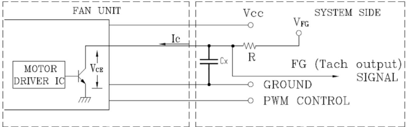
GENERAL CONDITION:  $V_{FG}$  is 3.3V,  $R$  is 8.2Kohm, and  $C_x$  is 4nF.
