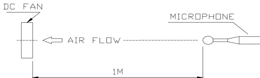
NOISE IS MEASURED AT RATED VOLTAGE IN FREE AIR IN ANECHOIC CHAMBER WITH B & K SOUND LEVEL METER WITH MICROPHONE AT A DISTANCE OF ONE METER FROM THE FAN INTAKE.
