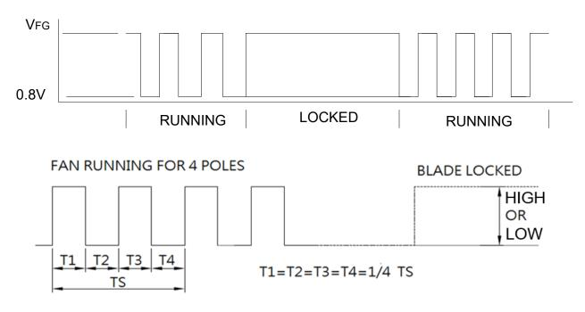
N=R.P.M TS=60/N(SEC) \*VFG IS ALWAYS HIGH OR LOW LEVEL AFTER BLADE LOCKED \*4 POLES
