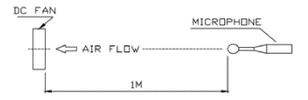
NOISE IS MEASURED AT RATED VOLTAGE IN FREE AIR IN SEMI-ANECHOIC CHAMBER WITH MICROPHONE AT A DISTANCE OF ONE METER FROM THE FAN INTAKE.
