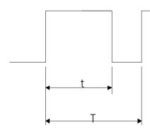
HIGH SIGNAL: HIGH SIGNAL: 15 VDC MAX. 3.3 VDC MIN. 0.8 VDC MAX. 0 VDC MIN.DUTY CYCLE=  $\frac{t}{T}$  \*100(%)
