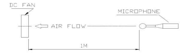
NOISE IS MEASURED AT RATED VOLTAGE IN FREE AIR IN SEMI-ANECHOIC CHAMBER WITH MICROPHONE AT A DISTANCE OF ONE METER FROM THE FAN INTAKE.
