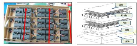
12-3-2. MAKE SURE DESICCANT, QUANTITY AND P/N IS CORRECT BEFORE PACKING.
