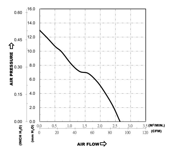
\*TEST CONDITION: INPUT VOLTAGE-----OPERATION VOLTAGE
