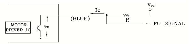
CAUTION: THE FG SIGNAL LEAD WIRE MUST BE KEPT AWAY FROM"+" LEAD WIRE & "-" LEAD WIRE.
