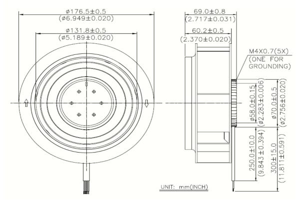
NOTES: 1. CABLE WIRE UL:2464 AWG#22 RED WIRE ----(+) YELLOW WIRE ----(PWM) BLUE WIRE ----(F00) BLACK WIRE ----(-)
