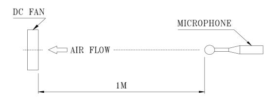
NOISE IS MEASURED AT RATED VOLTAGE IN FREE AIR IN ANECHOIC CHAMBER WITH MICROPHONE AT A DISTANCE OF ONE METER FROM THE FAN INTAKE.
