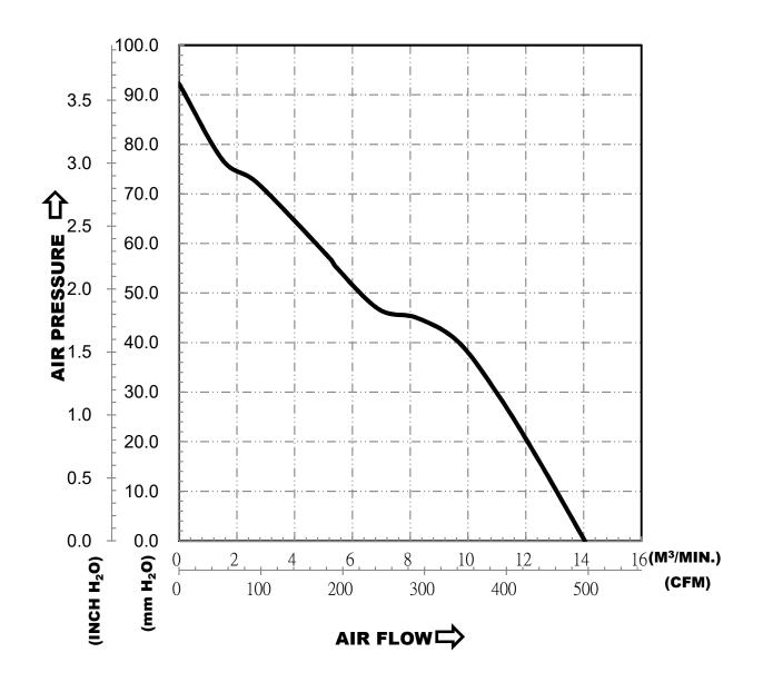
\*TEST CONDITION: INPUT VOLTAGE-----OPERATION VOLTAGE
