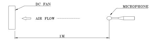
NOISE IS MEASURED AT RATED VOLTAGE IN FREE AIR IN ANECHOIC CHAMBER WITH MICROPHONE AT A DISTANCE OF ONE METER FROM THE FAN INTAKE.
